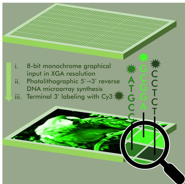
**Fig. 1** Schematic representation of the DNA painting process by microarray photolithography. A graphical input, in monochrome and of 1024 × 768 maximum resolution, is transformed into a Cy3-labelled DNA microarray. Colour intensity at the graphical level has a sequence equivalent and employs the sequence-dependent property of Cy3 fluorescence. DNA synthesis takes place using *in situ* microarray photolithography in the 5' → 3' direction, followed by terminal 3'-labeling with Cy3.
