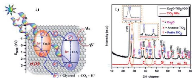
Fig. 27 (a) Representation of the Cu<sub>2</sub>O–TiO<sub>2</sub>/RGO water splitting reaction mechanism. (b) X-ray diffraction data of pristine TiO<sub>2</sub> nanoparticles and Cu<sub>2</sub>O–TiO<sub>2</sub>/RGO photocatalysts.<sup>103</sup> Copyright 2015, Nanoscale.
