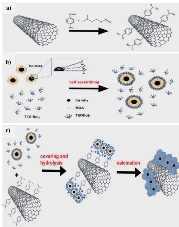
Fig. 21 Schematic representation of hierarchical CNTs/Pd-TiO<sub>2</sub> and CNTs/Pd-TiO<sub>2</sub>-calcination. (a) Covalent functionalization of the MWCNTs with benzoic acid of *in situ* made diazonium salt *via* radical addition. (b) Pd-TiO<sub>2</sub> precursor self-assembly mechanism. (c) Hydrolysis for obtaining the final material, fresh and calcined.<sup>98</sup> Copyright 2016, Green Chemistry.
