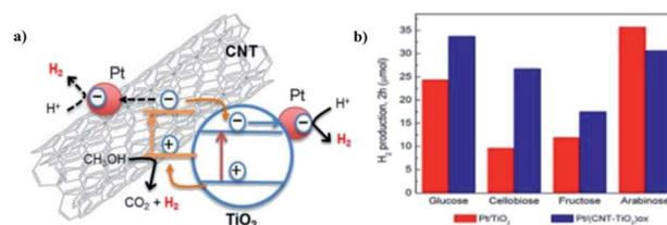
Fig. 24 (a) Scheme for the photocatalytic mechanism of  $\text{H}_2$  generation from water/methanol solutions by the  $\text{Pt}/(\text{CNT}-\text{TiO}_2)_{\text{ox}}-473$  catalyst using near UV-visible radiation. (b)  $\text{H}_2$  produced from saccharides (0.02 M) with  $\text{Pt}/\text{TiO}_2$  and  $\text{Pt}/(\text{CNT}-\text{TiO}_2)_{\text{ox}}$  catalysts.<sup>100</sup> Copyright 2015, Applied Catalysis B: Environmental.
