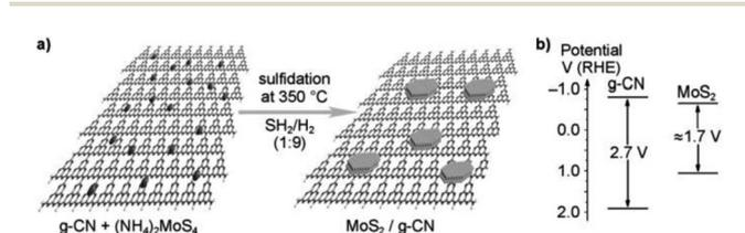
Fig. 29 (a) The theoretical structural model of the resultant MoS<sub>2</sub>/g-carbon nitride layered junctions and the process for gas-phase sulfidation. (b) g-CN and MoS<sub>2</sub> band gap energy diagram.<sup>105</sup> Copyright 2013, Angewandte Chemie.
