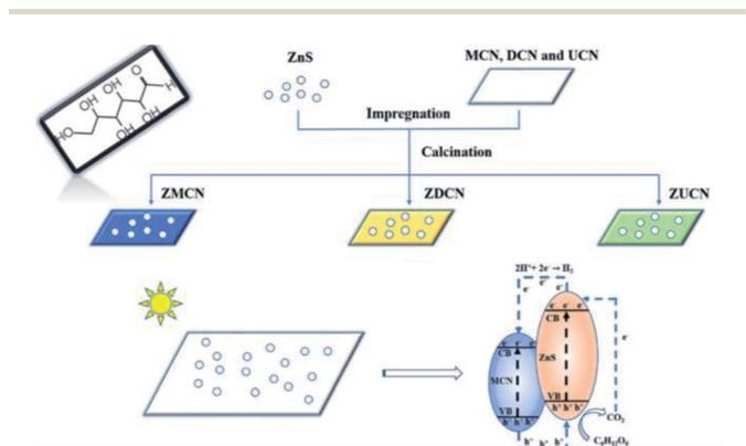
Fig. 13 Mechanism of photocatalytic reforming of glucose on  $ZnS/C_3N_4$ .<sup>90</sup> Copyright 2019, Journal of Colloid and Interface Science.
