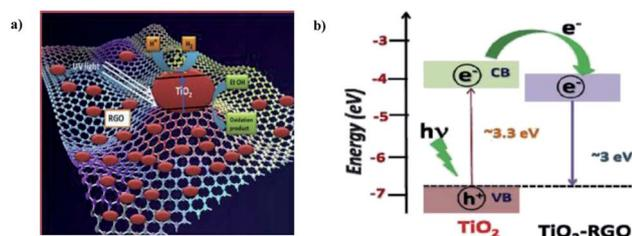
Fig. 25 (a) Representation of the photocatalytic hydrogen production from TiO<sub>2</sub>-RGO-based photocatalyst mechanism. (b) Energy level diagram of TiO<sub>2</sub> and RGO.<sup>101</sup> Copyright 2015, International Journal of Hydrogen Energy.
