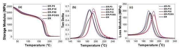
Fig. 5 Temperature plots of (a) storage modulus, (b) loss factor tan  $\delta$ , and (c) loss modulus of the neat and modified epoxy resins
