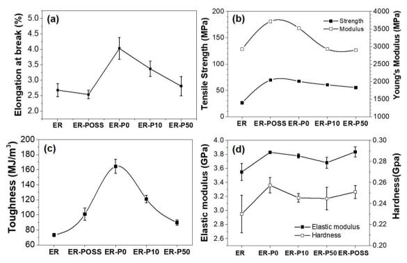
Plots of (a) elongation at breaks, (b) tensile strength, (c) toughness and (d) hardness for the neat and modified epoxy resins.
