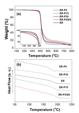
Fig. 4 (a) TGA and (b) DSC curves of the neat and modified epoxy resins.
