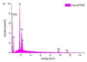
Fig. 2 a) IR spectra of Pine, Pine-NaOH and Pine-MA. b) EDXspectrum of Pine-APTES.
