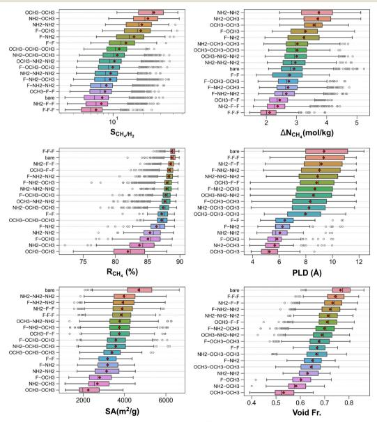
Fig. 4 CH<sub>4</sub>/H<sub>2</sub> separation performance metrics and structural properties of MOFs classified by their functional groups.
