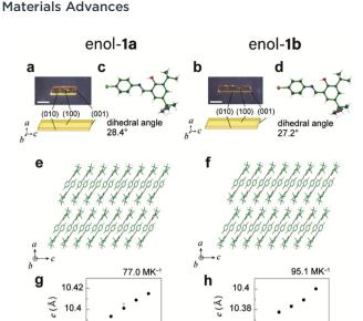
Fig. 1 Crystal structures of the enol-1a and enol-1b crystals. (a and b) Photographs and face indices of single plate-like (a) enol-1a and (b) enol-1b crystals. Scale bars, 1 mm. (c and d) Oak Ridge Thermal Ellipsoid Plot (ORTEP) drawings at 20 °C with a thermal ellipsoid of 25% probability. Disordered tert-butyl substituents are indicated in magenta. (e and f) Molecular packing on the (010) side face. (g and h) Temperature dependence of the length of the c-axis.
