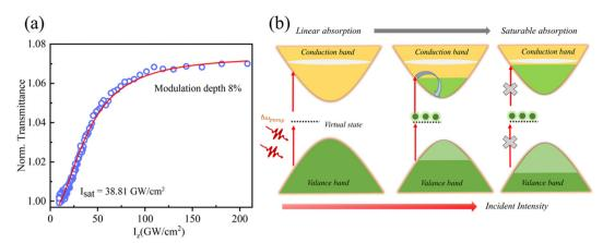
Fig. 5 (a) Normalised transmission as a function of intensity for 208 GW cm<sup>-2</sup>. (b) Schematic sketch of the mechanism behind SA in the sample.
