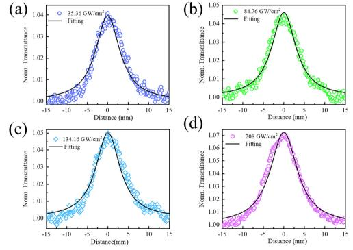
Fig. 4 Open aperture (OA) Z-scan curves obtained at an excitation wavelength of 800 nm for (a) 35.36, (b) 84.76, (c) 134.16 and (d) 208 GW cm<sup>-2</sup> input intensities. The solid line in each figure represents the fitting of experimental data.
