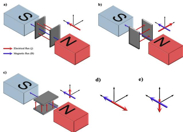
**Fig. 12** A schematic of the possibilities of orientation of electrode configuration with respect to the electromagnets and the consequent electrical and magnetic flux directions with its representation indicated as (a) parallel, (b) perpendicular, (c) perpendicular aligned against gravity, (d) antiparallel and (e) perpendicular aligned with gravity.
