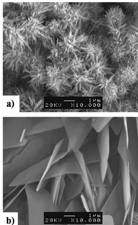
Fig. 15 SEM depicting the formation of (a) needle-like HAp in a N<sub>2</sub> atmosphere and (b) plate-like HAp in a CO<sub>2</sub> atmosphere electrodeposited under galvanostatic conditions. Adapted from ref. 152 with permission from Elsevier.
