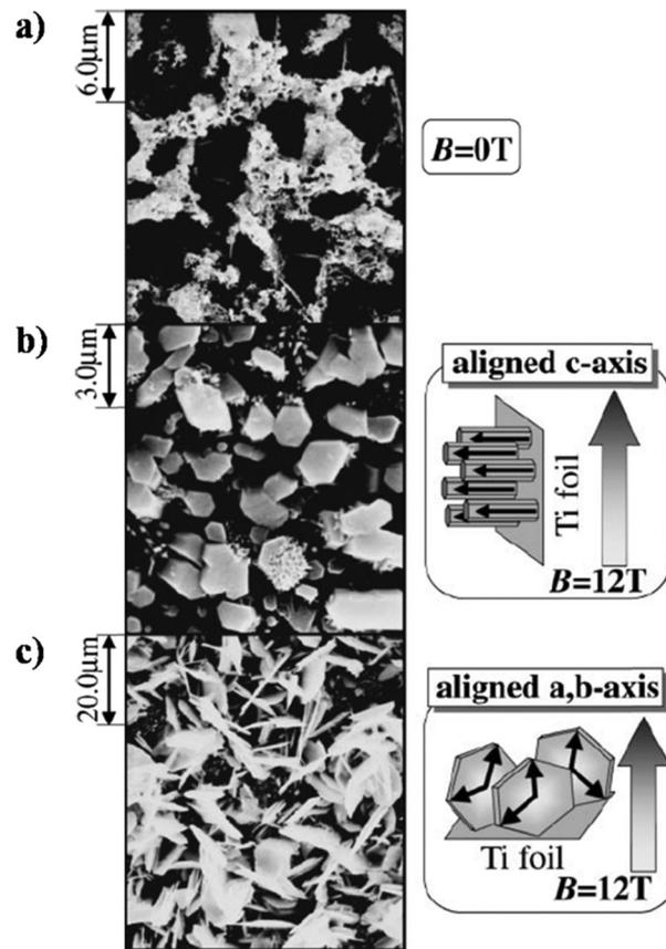
Fig. 11 SEM images of HAP electrodeposited via the heat substrate method over Ti foil under a magnetic field strength of (a)  $B = 0$ , (b)  $B = 12$  T ( $B \perp j$ ) and (c)  $B = 12$  T ( $B \parallel j$ ). Reproduced from ref. 124 with permission from The Japan Institute of Metals and Materials.
