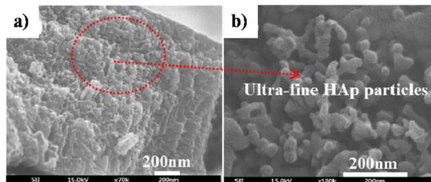
Fig. 8 FESEM of (a) HAp electrodeposited over TiO<sub>2</sub> NTs via the simultaneous anodization–electrodeposition technique and (b) the microstructure of the deposited HAp particles. Adapted from ref. 117 with permission from Elsevier.
