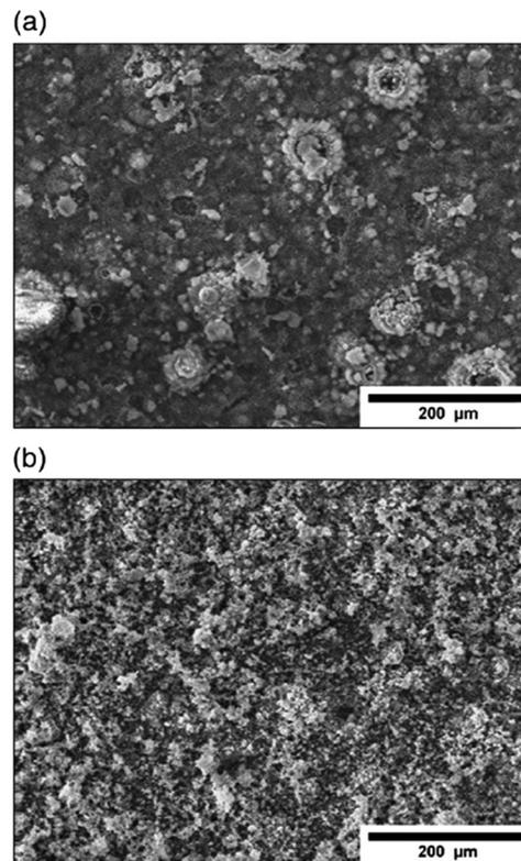
Fig. 7 SEM micrographs depicting electrodeposited HAP in a H<sub>2</sub>O<sub>2</sub> electrolytic environment under the (a) direct current method and (b) pulsed current method. Adapted from ref. 111 with permission from Elsevier.
