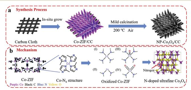
Fig. 14 Schematic demonstration of (a) the fabrication process of NP-Co<sub>3</sub>O<sub>4</sub>/CC and (b) the proposed mechanism of nitrogen doping in cobalt oxide lattices. Reproduced from ref. 282 with permission from Elsevier B.V.
