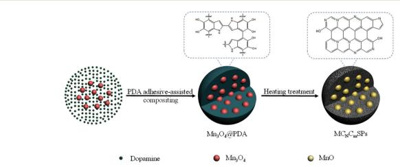
Fig. 8 Schematic illustration of the fabrication of MCNCmSPs by a PDA adhesive-assisted compositing procedure. Reproduced from ref. 177 with permission from Elsevier Ltd.
