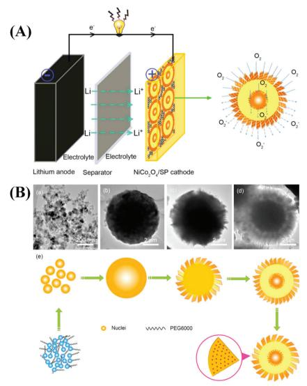
Fig. 10 (A) Representative schematic illustration of the Li-O<sub>2</sub> battery catalyzed by 3D porous NiCo<sub>2</sub>O<sub>4</sub> core-shell microspheres. (B) Time-dependent experiment of NiCo<sub>2</sub>O<sub>4</sub> at different reaction times: (a) 1 h, (b) 3 h, (c) 5 h, and (d) 10 h, and (e) the corresponding scheme of the reaction process. Reproduced from ref. 239 with permission from Elsevier Ltd.
