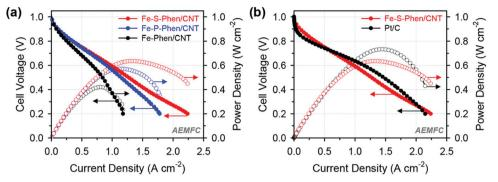
Fig. 5 Alkaline AEMFC performance of MEAs using (a) Fe-Phen/CNT, Fe-P-Phen/CNT, and Fe-S-Phen/CNT as cathode catalysts and (b) Fe-S-Phen/CNT. CNT and Pt/C as cathode catalysts. Reproduced from ref. 76 with permission from the American Chemical Society
