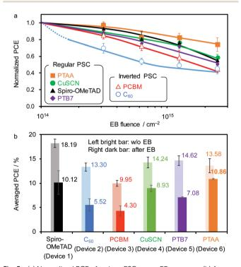
Fig. 5 (a) Normalized PCE of various PSCs upon EB exposure. (b) Average PCE values with error bars (standard deviation) before (left bar) and after EB (right bar,  $F_{EB} = 2.5 \times 10^{15} \text{ cm}^{-2}$ ) exposure.
