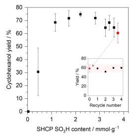
Fig. 4 Cyclohexanol yield of SHCP catalysed hydrolysis of cyclohexyl acetate as a function of  $\rm SO_3H$  content. The inset shows the catalytic performance of recycled SHCP-10 in the same conversion over four cycles.
