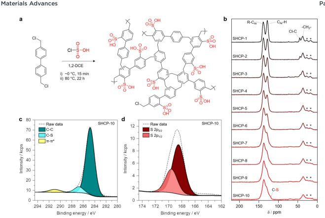
Fig. 1 Sulfonated hypercrosslinked polymer characterisation. (a) Reaction scheme for the one-pot synthesis of SHCPs. (b) <sup>13</sup>C CP/MAS solid state NMR spectra for all SHCPs, with increasing catalyst to monomer ratio used in the production of SHCP-1-SHCP-10. \* Represents spinning side bands. (c) X-Ray photoelectron C 1s spectrum for SHCP-10. (d) X-Ray photoelectron S 2p spectrum for SHCP-10. (grey dotted lines in (c and d) represent raw data).
