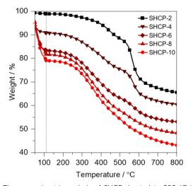
Fig. 3 Thermogravimetric analysis of SHCPs heated to 800 °C in a N<sub>2</sub> atmosphere. A 10 min isothermal step was included at 110 °C to remove residual water (indicated by the vertical grey dotted line)
