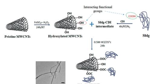
Fig. 7 The preparation process of succinylated β-lactoglobuline-functionalized MWCNTs. CDI: N,N'-carbonyldiimidazole, Sblg: succinylated β-lactoglobuline. Reproduced with permission from ref. 170 Copyright 2019 American Chemical Society.
