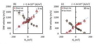
Fig. 6 (a) The estimated temperature profile calculation results of the cross-section of the magnetic wire due to the Joule heat when a pulse current was applied to the magnetic wire. The orange dot shows the result of the pulse current application time of 30 ns, and the blue dot shows that of 3 ns. Domain wall (DW) velocity as a function of an external in-plane field  $(H_x)$  along the wire for (b) 3 ns and (c) 30 ns pulse duration width.
