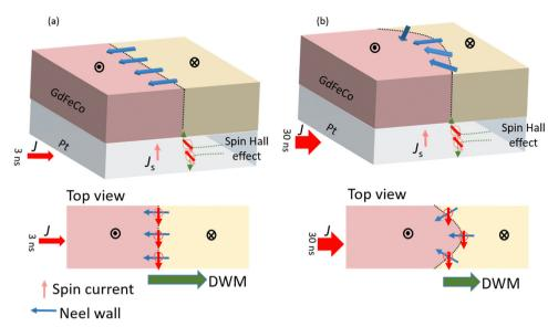
Fig. 5 Schematic illustration of the domain wall (DW) shape for (a) 3 ns and (b) 30 ns pulse duration width.
