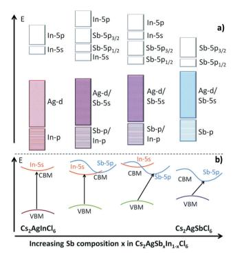
Fig. 10 (a) Schematic diagram of the bonding and antibonding orbitals of Cs<sub>2</sub>AgSb<sub>x</sub>In<sub>1-x</sub>Cl<sub>6</sub> and (b) transition from direct to indirect bandgaps on changing the character of the VBM and CBM. Reproduced with permission.90 Copyright 2017, Royal Society of Chemistry.
