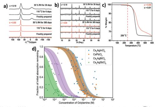
Fig. 16 (a) NMR, (b) P-XRD and (c) TGA spectra of undoped and Cu doped  $Cs_2AgSbCl_6$  MCs. Reproduced with permission. Reproduced with permission. Chemical Society. (d) Stability analysis of Cs<sub>2</sub>AgSbCl<sub>6</sub>, Cs<sub>2</sub>AgInCl<sub>6</sub>, Cs<sub>2</sub>AgBiCl<sub>6</sub> and CsPbCl<sub>3</sub> NCs by amine titration. Reproduced with permission. 83 Copyright 2019, American Chemical Society.
