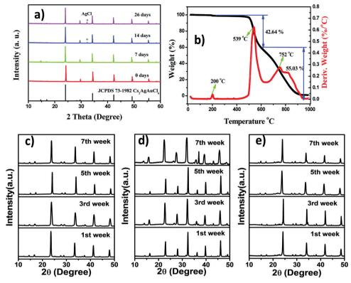
Fig. 15 Cs<sub>2</sub>AgInCl<sub>6</sub> MCs: (a) P-XRD patterns at 7, 14 and 26 day intervals, and (b) TGA and DSC curves. Reproduced with permission.<sup>79</sup> Copyright 2017, Royal Society of Chemistry. P-XRD patterns of (c) Cs<sub>2</sub>AgBiCl<sub>6</sub> MCs and (d) Cs<sub>2</sub>AgBiBr<sub>6</sub> MCs in organic medium, and (e) Cs<sub>2</sub>AgBiBr<sub>6</sub> MCs in a mixture of aqueous and organic media. Reproduced with permission.<sup>76</sup> Copyright 2021, Elsevier.
