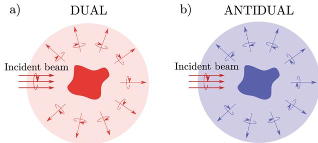
Fig. 2 (a) A sketch of a generic dual sample, *i.e.* a scatterer which preserves the helicity of an incident electromagnetic field; (b) a sketch of a generic antidual sample, *i.e.* a scatterer which flips the helicity of an incident electromagnetic field. Red and blue arrows represent circularly polarized planewaves with opposite helicities.
