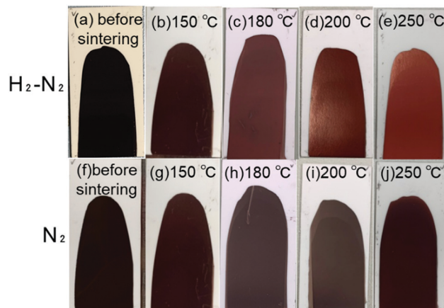
Fig. 7 Digital images of the surface of the sintered copper nanoparticle layers. (a) Before sintering, (b–e) sintered at various temperatures indicated in the image under 3%H 2 -N 2 gas flow, (f) before sintering, (g–j) sintered at various temperatures under nitrogen gas flow.
