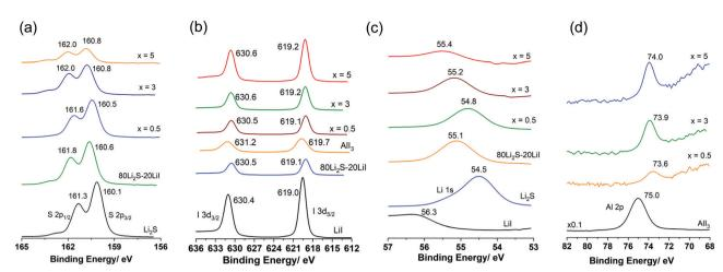
X-Ray photoelectron spectroscopy spectra (envelope) of the prepared samples and standard materials. (a) S 2p; (b) I 3d; (c) Li 1s; and (d) Al 2p.
