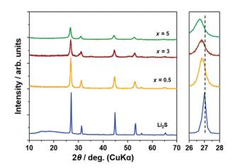
Fig. 1 X-Ray diffraction patterns of  $(100 - x)Li_2S \cdot xAll_3$  and a magnified
