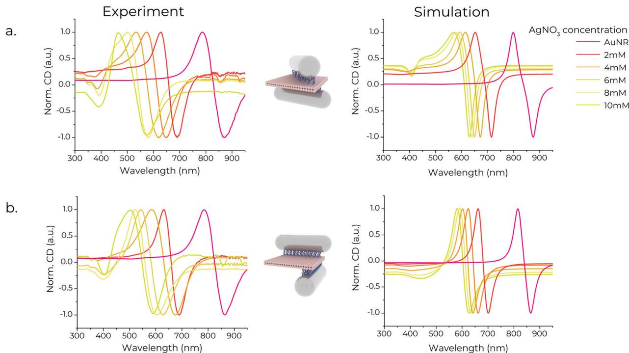
Fig. 4 Experimental (left) and theoretically calculated (right) CD spectra of the (a) X-shaped and (b) L-shaped chiral metamolecules constructed using Au/AgNRs with Ag shells of varying thicknesses. The legend shows the concentration of  $\text{AgNO}_3$  used to synthesise the nanorods in the metamolecules.
