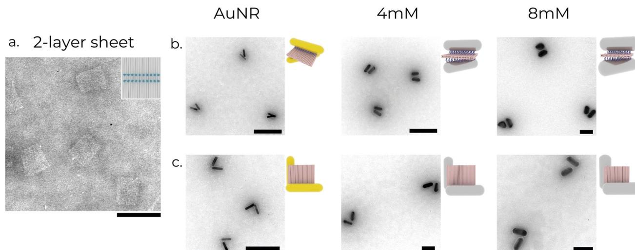
Fig. 3 Structural characterisation of chiral metamolecules. (a) Transmission electron micrograph of the 2-layer sheet DNA origami structures. (b) and (c) X- and L-shaped left-handed chiral structures assembled using three varieties of nanorods, respectively. The concentration of  $\text{AgNO}_3$  used to synthesise the nanorods used for the structures is shown above the images. All scale bars: 100 nm.
