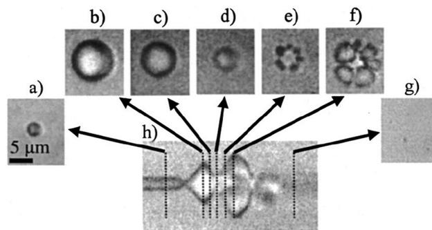
Fig. 2 Optical frame (a–g) and streak (h) images showing the oscillation and fragmentation of an ultrasound contrast agent microbubble. The microbubble has an initial diameter of 3  $\mu\text{m}$  (a), and the streak image (h) shows the changes in the bubble diameter as a function of time and the ultrasound pressure wave, with the fragmentation occurring during compression (e and f). Reprinted with permission from ref. 53.
