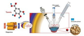
Fig. 5 Schematic illustration of the experimental setup for ultrasound/microwave-assisted extraction (UMAE) of tannin.
