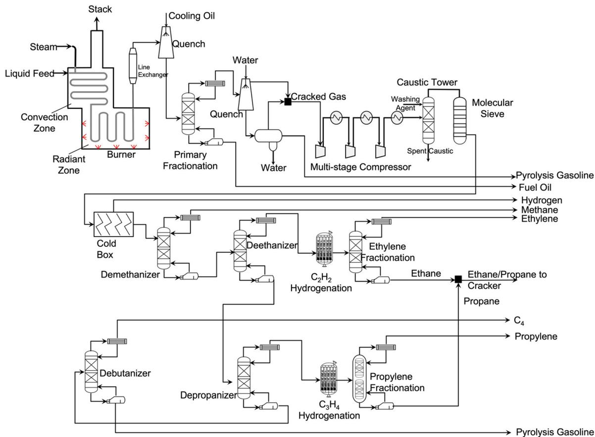
Fig. 4 A simplified process flowsheet diagram of steam cracking.<sup>27–29</sup>
