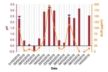
Fig. 3 Aerosol liquid water (ALW) content and aerosol pH calculated using the model E-AIM IV based on the bulk chemical composition of  $PM_{2.5}$ , and average RH and T over the 24 h sampling period. The blue triangles indicate the days with observed fog formation.
