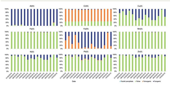
Fig. 5 Speciation of soluble metals ( $t = \infty$ ) in simulated fog (T = 5 °C, pH = 4.7) obtained using the model Visual MinteQ.
