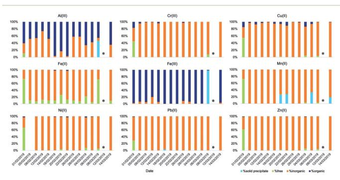
Fig. 4 Speciation of readily soluble metals (t = 2 min) in ALW obtained using the model Visual MinteQ.
