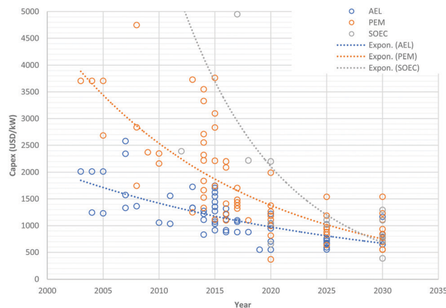
Fig. 6 Examples of CAPEX estimates for different electrolyser types for the year of development. Source: Glenk & Reichelstein. 155
