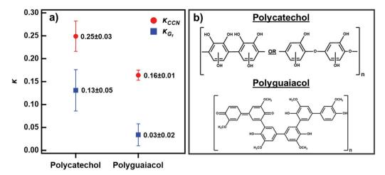
Fig. 4 (a) The average  $\kappa_{\text{CCN}}$  (red circles) and  $\kappa_{\text{G}}$ , (blue circles) of polycatechol and polyguaiacol. Error bars represent standard deviation. (b) The chemical structures of polycatechol and polyguaiacol adapted from Al-Abadleh.<sup>14</sup>
