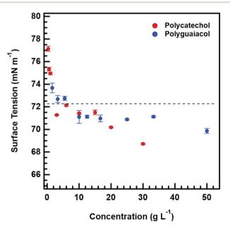
Fig. 5 Surface tension measurements for polycatechol (red circles) and polyguaiacol (blue circles). Horizontal line represents pure water,  $ST = 72.27 \text{ mN m}^{-1}$ . Room temperature: 21.8 °C. Error bars represent standard deviation.
