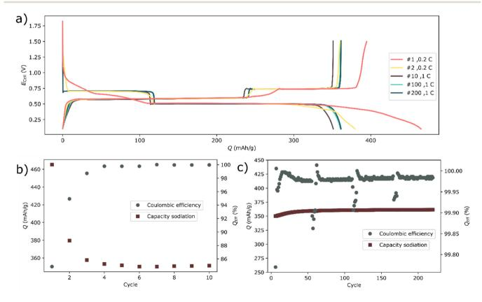
Fig. 1 (a) The voltage profile of a bismuth half-cell. (b) The capacity during sodiation (discharging) and coulombic efficiencies during the first 10 cycles and (c) 6 to 220 cycles.
