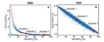
Fig. 5 (a) Intensity ratio between  $011_R$  and  $011_\beta$  lines from the modelled XRD patterns plotted against the β-MnO<sub>2</sub> fraction (%β-MnO<sub>2</sub>, blue dots) and fitted using eqn (3) (red solid line). (b) Intensity ratio between PDF peaks at 2.8 Å and 3.4 Å from the modelled PDFs plotted against  $\%\beta$ -MnO<sub>2</sub> (blue dots) and fitted using a linear function (red solid line).
