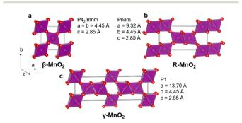
Fig. 1  $\beta$ -MnO<sub>2</sub> (a) and R-MnO<sub>2</sub> (b) can randomly be stacked along their common *a*-axis to form an intergrowth  $\gamma$ -MnO<sub>2</sub> structure (c).
