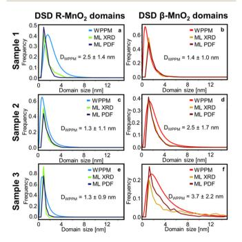
Fig. 8 Domain Size Distributions (DSD) determined by Whole Powder Pattern Modelling (WPPM), ML-MotEx analysis of XRD (ML XRD) and PDF (ML PDF) refinement results of R- and  $\beta$ -MnO<sub>2</sub> domains in samples 1 (a and b), 2 (c and d) and 3 (e and f).
