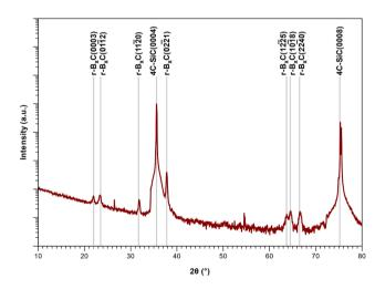
**Fig. 6**  $2\theta/\omega$  diffractogram of a polycrystalline B<sub>x</sub>C deposited at 1400 °C close to the inlet of the susceptor, corresponding to a residence time of 0.06 s. The sharp low-intensity non-indexed peaks come from the substrate.
