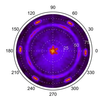
Fig. 8 Pole figure of the r-B<sub>x</sub>C{1014} plane family ( $2\theta = 35.08^{\circ}$ ,  $\psi = 60^{\circ}$ ) of a r-B<sub>x</sub>C film deposited at 1400 °C on 4H-SiC(0001), showing a five-fold pattern and its orientation with respect to the substrate (4H-SiC {1011} at  $2\theta = 34.84^{\circ}$ ,  $\psi = 75.17^{\circ}$ ). The strong pole at the center originates both from r-B<sub>x</sub>C{1014} and the tail of 4H-SiC(0001) ( $2\theta = 35.6^{\circ}$ ,  $\psi = 0^{\circ}$ ).
