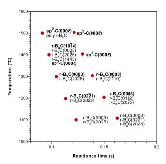
Fig. 7 Evolution of the orientation, from  $2\theta/\omega$  XRD, of the r-B<sub>x</sub>C films deposited on 4H-SiC(0001) substrates placed at the center and the backside of the susceptor. Bold face marks the dominating orientations. The corresponding residence times and temperatures were estimated by modeling.
