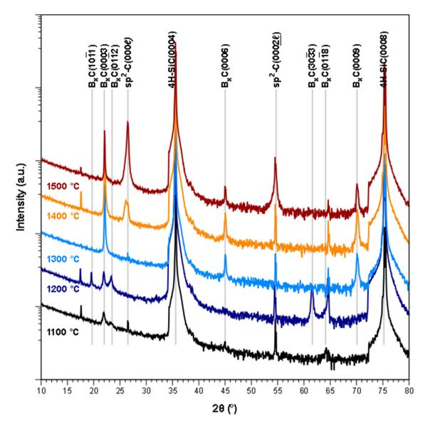
Fig. 1 XRD 2θ/ω diffractograms of r-B<sub>x</sub>C films deposited on 4H-SiC(0001) at temperatures (from bottom to top) of 1100, 1200, 1300, 1400 and 1500 °C. The low intensity, non-indexed sharp peaks are the forbidden 4H-SiC(000ℓ) diffraction peaks.
