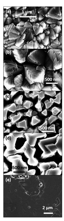
Fig. 4 Plan view SEM of rhombohedral boron carbide deposited on 4H-SiC(000 $\bar{1}$ ); at (a) 1100 °C, (b) 1200 °C, (c) 1300 °C, (d) 1400 °C and (e) 1500 °C.
