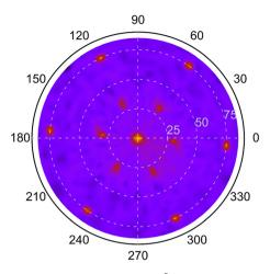
Fig. 2 X-ray pole figure of the r-B<sub>x</sub>C{ $10\overline{1}4$ } plane family ( $2\theta = 35.08^{\circ}$ ,  $\psi$  = 31.81°) of a r-B<sub>v</sub>C film deposited at 1300 °C on 4H-SiC(0001), showing the epitaxial relationship with the substrate (4H-SiC{1011}) at  $2\theta$  = 34.84°,  $\psi$  = 75.17°) and rotational twinning. The strong pole at the center originates from the tail of 4H-SiC{0001} ( $2\theta = 35.6^{\circ}$ ,  $\psi = 0^{\circ}$ ).
