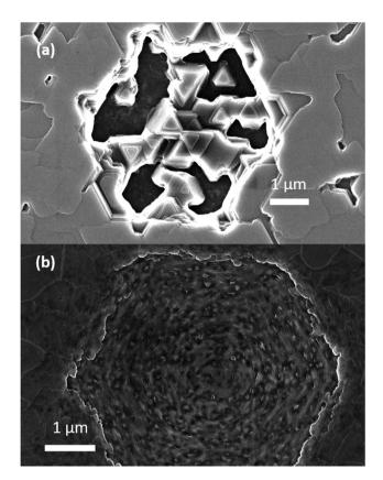
Fig. 5 Plan view SEM of the defects observed (a) rhombohedral boron carbide film and (b) pyrolytic graphite co-deposited at 1500  $^{\circ}$ C on 4H-SiC(000 $\bar{1}$ ).
