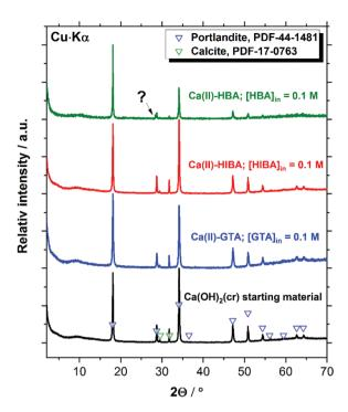
Fig. 7 XRD patterns of the Ca(II) solid phase used as starting material, and the corresponding solid phases after equilibration in the solubility experiments with GTA, HIBA and HBA at  $[L]_{tot} = 0.1$  M. Symbols reproduce the patterns reported for portlandite (Ca(OH)<sub>2</sub>(cr), PDF-44-1481) and calcite (CaCO<sub>3</sub>(cr), PDF-17-0763) reference materials.
