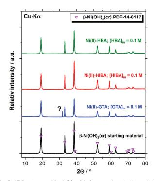
Fig. 8 XRD patterns of the Ni(II) solid phase used as starting material, and the corresponding solid phases after equilibration in the solubility experiments with GTA, HIBA and HBA at  $[L]_{tot} = 0.1$  M. Symbols reproduce the patterns reported for  $\beta$ -Ni(OH)<sub>2</sub>(cr) (PDF-14-0117) reference material
