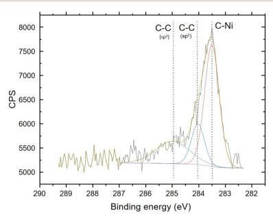
Fig. 9 The C 1s XPS spectrum of the 35 nm thick Ni film deposited at 110 °C. The fitted peaks correspond to the different types of carbon bonds and the clearly dominant peak is attributed to the C–Ni bond.
