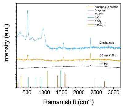
Fig. 10 Raman spectra from a 35 nm Ni film deposited at 110 °C and, for reference, from a nickel metal foil and the Si substrate. Band positions for selected phases are shown with bars. Carbon and  $NiCl_2$  band positions are from Wu et al.<sup>32</sup> and Lockwood et al.<sup>34</sup> respectively. NiO and  $Ni(CO_3)$  band positions are determined from ROD 3500021 and RRUFF R040157 entries respectively.
