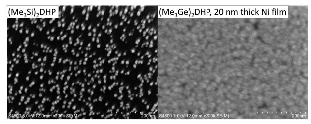
Fig. 3 Films deposited at 110 °C from NiCl<sub>2</sub>(PEt<sub>3</sub>)<sub>2</sub> and either (Me<sub>3</sub>Si)<sub>2</sub>DHP or (Me<sub>3</sub>Ge)<sub>2</sub>DHP. (With (Me<sub>3</sub>Si)<sub>2</sub>DHP only a layer of Ni islands was deposited, indicating a much lower growth rate at the same temperature.)
