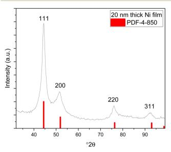
Fig. 5 Grazing incidence X-ray diffractogram of the 20 nm Ni film deposited at 110 °C.
