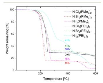
Fig. 2 TG curves measured for different  $NiX_2(PR_3)_2$  (X = Cl, Br, I; R = Me, Et) compounds.
