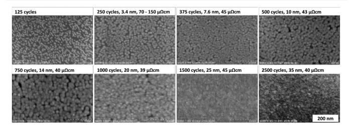
Fig. 6 SEM images of Ni films deposited at 110 °C with varying number of cycles with their respective thicknesses and resistivities.
