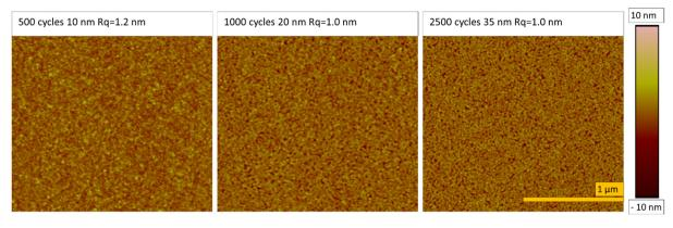
Fig. 7 AFM images taken of the Ni films deposited at 110 °C with varying number of cycles.
