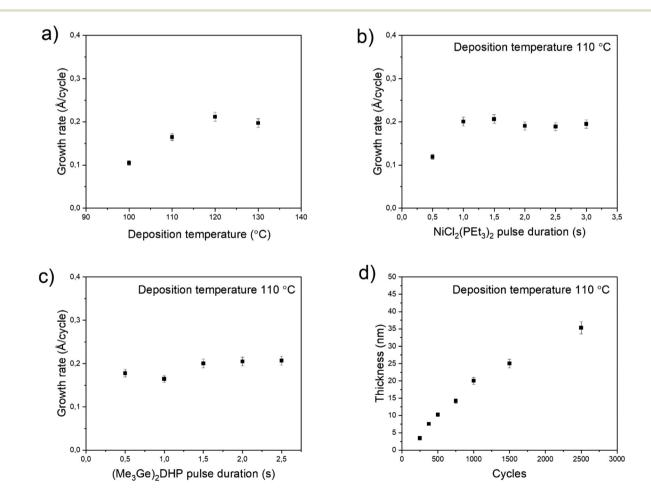
Fig. 4 Growth characteristics of the (Me<sub>3</sub>Ge)<sub>2</sub>DHP + NiCl<sub>2</sub>(PEt<sub>3</sub>)<sub>2</sub> process. The growth rate as a function of the deposition temperature (a), NiCl<sub>2</sub>(PEt<sub>3</sub>)<sub>2</sub> pulse length (b), and (Me<sub>3</sub>Ge)<sub>2</sub>DHP pulse length (c). Film thickness as a function of number of cycles (d).
