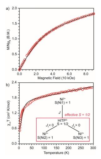
Fig. 3 (a) Field-dependent magnetization (T=1.8 K); (b) temperature-dependent  $\chi_{\rm m}T$  (H=1.0 kOe) curves for 1. Solid black lines are fits described in text. Inset: magnetic coupling scheme proposed for 1. The red box highlights two Ni atoms and the HITP ligand forming a single spin system with effective S=1/2.
