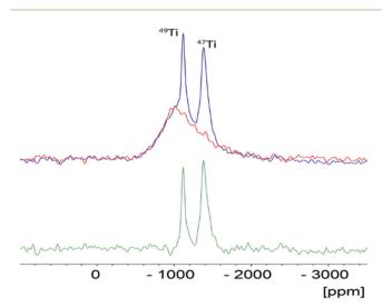
Fig. 9 Static titanium NMR spectra of TiP1-H (red) and LTP-H (blue), scaled to the same height, and their difference (green). The resonances from both titanium isotopes, <sup>49</sup>Ti and <sup>47</sup>Ti, are clearly resolved in the difference spectrum.
