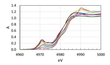
Fig. 6 Titanium K edge XANES spectra of titanium(IV) phosphates, sample 1 – TiP1-H, sample 2 –  $\alpha$ -TiP, sample 3 – LTP-H, sample 4 – a-TiP, sample 5 - LTP-Na sample 6 - LTP-pro, sample 7 - TiP1-Na and sample 9 - TiP1-mix and sample 10 - TiP1-mixCa (overlapping spectra samples 9 and 10), (sample 8 - no data available).
