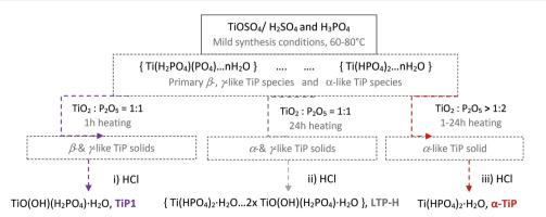
Scheme 1 Overall representation of suggested chemical changes during synthesis and post-washing steps with hydrochloric acid of different TiP materials, TiP1-H, LTP-H and  $\alpha$ -TiP.
