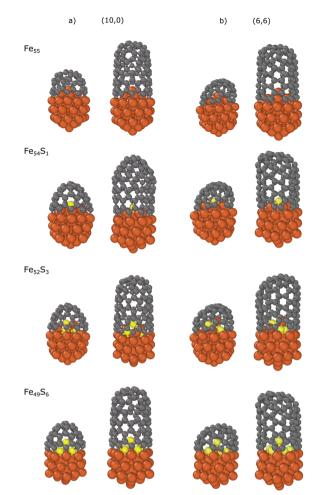
Fig. 5 Optimized structures of the carbon nanocaps and CNT segments with chirality indices of (a) (10,0) and (b) (6,6) binding to  $Fe_{55-x}S_x$ (x = 0,1,3,6) nanoparticles.
