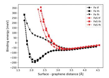
Fig. 2 Potential energy curves of graphene binding to the Fe (black lines) and sulfur covered FeS (red lines) surface with the fcc(111) arrangement in three different configurations: top-fcc (tf), top-hollow (th), and fcc-hollow (fh).
