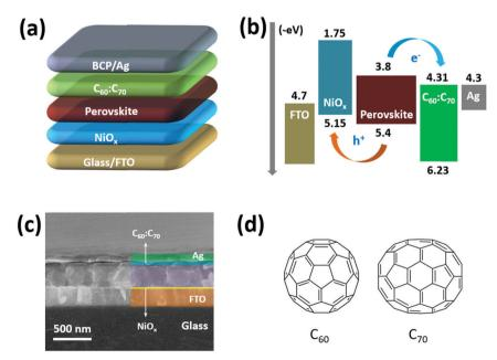
Fig. 1 (a) Schematic device structure of the PSCs; (b) schematic energy levels of the functional layers involved in the PSCs; (c) cross-sectional SEM image of a PSC; (d) molecular structures of  $C_{60}$  and  $C_{70}$
