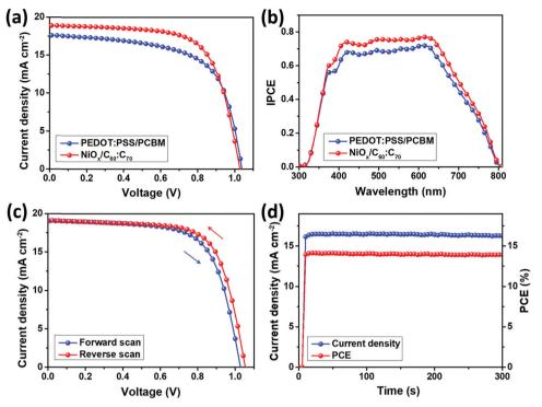
Fig. 2 Forward scanning J-V characteristics (a) and IPCE spectra (b) of the PSCs using PEDOT:PSS/PCBM and NiO<sub>x</sub>/C<sub>60</sub>: C<sub>70</sub> as the charge transport layers; (c) forward and reverse scanning J-V characteristics of a best performing PSC using NiO<sub>x</sub> and C<sub>60</sub>: C<sub>70</sub> as the HTL and ETL; and (d) current density and PCE as a function of time for the best performing PSC under a bias of 0.86 V.
