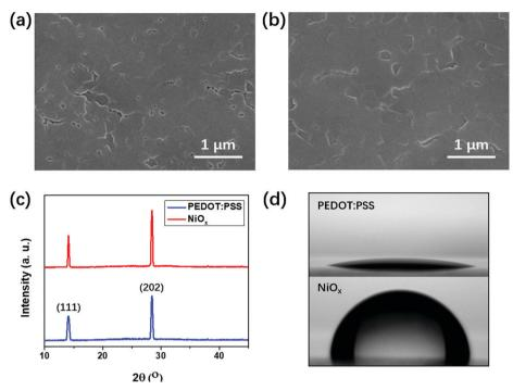
Fig. 3 SEM images of the  $(BA)_2(MA)_3Pb_4|_{13}$  perovskite films formed on (a) PEDOT:PSS and (b)  $NiO_x$ ; (c) XRD patterns of the perovskite films formed on PEDOT:PSS and  $NiO_x$ ; and (d) contact angles of water drops on the surfaces of PEDOT:PSS and  $NiO_x$  films.
