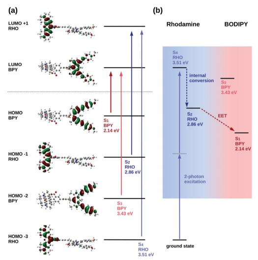
Fig. 3 (a) Frontier molecular orbitals involved in the excited electronic states of interest in RHO-BPY-OH. (b) Schematic illustration of the processes triggered by two-photon excitation of RHO-BPY-OH.
