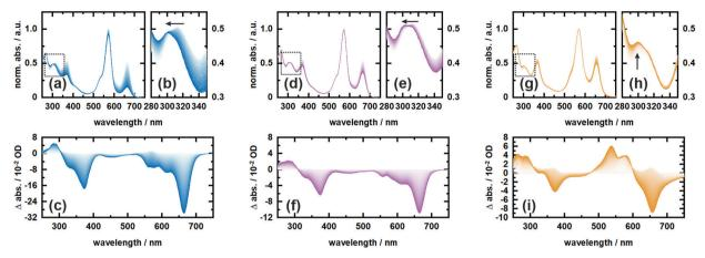
Fig. 4 Irradiation experiments of RHO-BPY-PNA (in MeOH) with 565 nm light (a-c) and 660 nm light (d-f), as well as irradiation of RHO-BPY-OH (in MeOH) with 565 nm light (q-i). (a), (d) and (g) depict the respective normalized spectra with a closer zoom in (b), (e) and (h) as indicated by the dashed boxes. (c), (f) and (i) show the respective difference spectra referenced to the initial dark measurement. The spectra were recorded in 30 s intervals in a total timeframe of 6000 s
