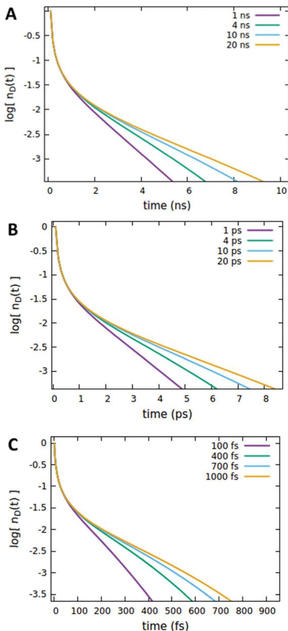
**Fig. 8** The effect of the quencher lifetime  $\tau_q$  on the (normalized) exciton density decay considering different timescales for the dye lifetime  $\tau_d$ , including (A) nanosecond ( $\tau_d = 4.242$  ns), (B) picosecond ( $\tau_d = 4$  ps), and (C) femtosecond ( $\tau_d = 400$  fs) timescales. Fixed parameters are  $R_{d+d} = 5$  nm;  $R_{d+d^*} = 4$  nm;  $R_{d+q} = 2$  nm;  $C_q = 0.25\%$  of  $C_d^{\text{TOT}}$ ;  $n_d(0) = 7\%$  of  $C_d^{\text{TOT}}$ .
