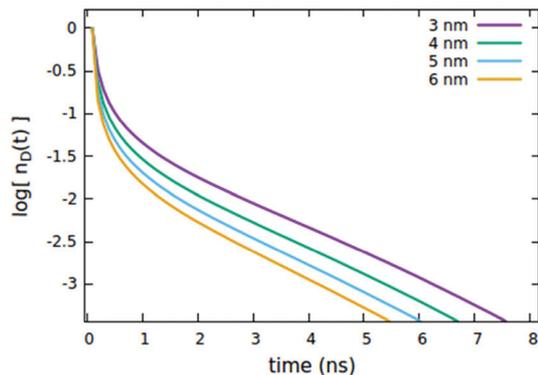
Fig. 4 Effect of the  $R_{d+d^*}$  radius governing the direct EEA mechanism on the (normalized) exciton density decay. Fixed parameters are  $R_{d+d^*} = 5$  nm;  $R_{d+q} = 2$  nm;  $\tau_q = 4$  ns;  $C_q = 0.25\%$  of  $C_d^{\text{TOT}}$ ;  $n_d(0) = 7\%$  of  $C_d^{\text{TOT}}$ .
