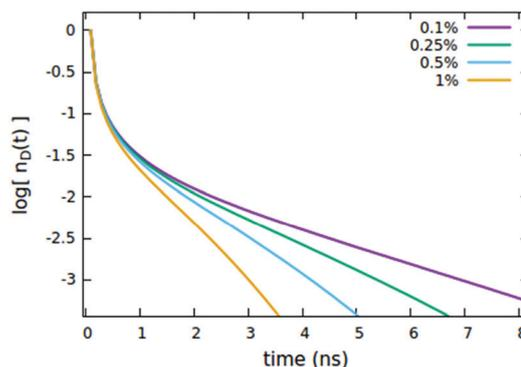
Fig. 7 Effect of the quencher concentration  $C_q$  (expressed as % of  $C_d^{\text{TOT}}$ ) on the (normalized) exciton density decay. Fixed parameters are  $R_{d+d^*} = 5$  nm;  $R_{d+d^*} = 4$  nm;  $R_{d+q} = 2$  nm;  $\tau_q = 4$  ns,  $C_q = 0.25\%$  of  $C_d^{\text{TOT}}$ ;  $n_d(0) = 7\%$  of  $C_d^{\text{TOT}}$ .
