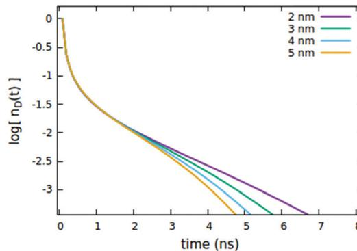
Fig. 6 Effect of the  $R_{d+q}$  radius governing the direct quenching mechanism on the (normalized) exciton density decay. Fixed parameters are  $R_{d+d^*} = 4$  nm;  $R_{d+d^*} = 5$  nm;  $\tau_q = 4$  ns;  $C_q = 0.25\%$  of  $C_d^{\text{TOT}}$ ;  $n_d(0) = 7\%$  of  $C_d^{\text{TOT}}$ .
