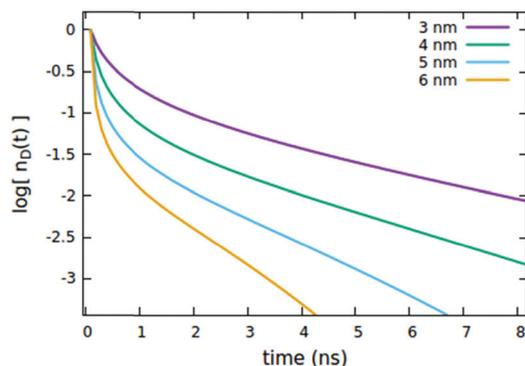
Fig. 5 Effect of the  $R_{d+d}$  radius governing both EEA and quenching diffusive mechanisms on the (normalized) exciton density decay. Fixed parameters are  $R_{d+d^*} = 4$  nm;  $R_{d+q} = 2$  nm;  $\tau_q = 4$  ns;  $C_q = 0.25\%$  of  $C_d^{\text{TOT}}$ ;  $n_d(0) = 7\%$  of  $C_d^{\text{TOT}}$ .
