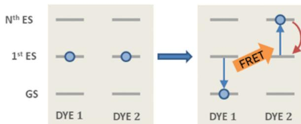
**Fig. 1** The mechanism for exciton–exciton annihilation (EEA). The excitation is transferred between two excited dyes (DYES 1 and 2), leading to an excited state absorption (to the  $N$ th excited state) in one dye (DYE 2) and to a relaxation to the ground state in the other one (DYE 1). The  $N$ th high-lying state is expected to rapidly decay non-radiatively (red arrow) to the first excited state, leading to the annihilation of one excitation (*i.e.* that of DYE 1).
