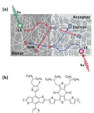
Fig. 1 (a) Simplified illustration of photophysical processes in bulkheterojunction organic photovoltaic devices. In both donor and acceptor domains, when locally excited (LE) states are generated upon photoexcitation, the LE states diffuse to the donor-acceptor interface and form charge-transfer state (CT). The CT state dissociates across the donoracceptor interface into charge-separated states. (b) Chemical structure of PM6
