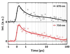
Fig. 5 Fluorescence-upconversion spectroscopy of PM6 in CHCl<sub>3</sub>.  $M_{\rm n} = 40.3$  kDa. [PM6] = 15  $\mu$ g mL<sup>-1</sup>. Excitation wavelength is 570 nm. Photoluminescence wavelengths are given in the panels. Multiexponential fits are given in solid lines.
