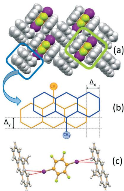
Fig. 3 Packing features of (MA)<sub>4</sub>·I2F4 showing (a) the I2F4 molecules “sandwiched” between MA molecules (lime rectangle) and the  $\pi$ -stacked MA pairs (blue rectangle), (b) details of the head-to-tail pair arrangement ( $\Delta y$  and  $\Delta x$  indicate the transversal and longitudinal offsets, respectively), and (c) the geometry of the I... $\pi$  interactions.
