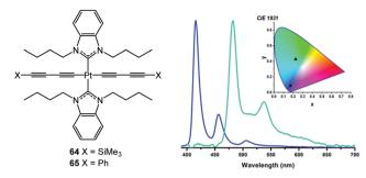
Fig. 24 Structures of 64 and 65, and EL spectra of PhOLEDs of 64 (blue) and 65 (green). Reproduced with permission from ref. 175 with permission from the American Chemical Society.
