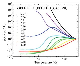
Fig. 3 DC resistivity of  $\kappa$ -[(BEDT-TTF)<sub>1-x</sub>(BEDT-STF)<sub>x</sub>]<sub>2</sub>Cu<sub>2</sub>(CN)<sub>3</sub> for various substitution values x measured as a function of temperature along the highly conducting c-axis and normalized to the room-temperature values. The substitution spans the full range from the insulating x = 0 to the metallic side
