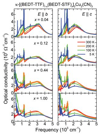
Fig. 4 Frequency dependent conductivity of  $\kappa$ -[(BEDT-TTF)<sub>1-x</sub>  $(BEDT-STF)_x]_2Cu_2(CN)_3$  for several substitution values x = 0.04, 0.12, 0.44, and x = 1 recorded for the two polarizations within the plane (left column  $E \parallel b$ ; right column  $E \parallel c$ ) at different temperatures as indicated in the legend.
