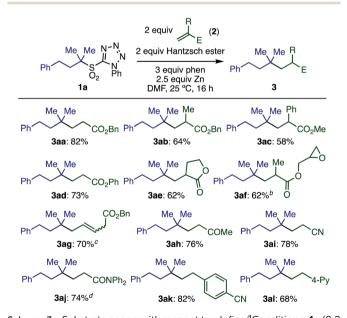
Scheme 3 Substrate scope with respect to olefins. Conditions: 1a (0.2 mmol), 2a (2 equiv.), Hantzsch ester (2 equiv.), phen (3 equiv.), Zn (particle size < 10  $\mu$ m, 2.5 equiv.), DMF (0.2 M), 25 °C, 16 h.  $^b$ 1 : 1 ratio of diastereomers.  $^{c}trans$ : cis = 17:1.  $^{d}50$   $^{\circ}C$ .
