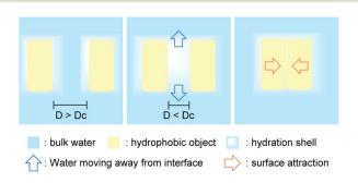
Fig. 4 Hydrophobic effect leading to the merging of two hydrophobic entities.
