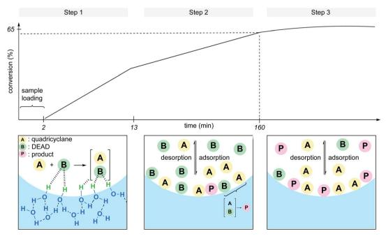
Interface adsorption/desorption in micro-droplets.
