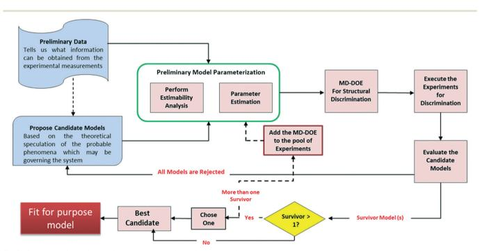
Fig. 1 Proposed scheme for kinetic model structure identification and development.
