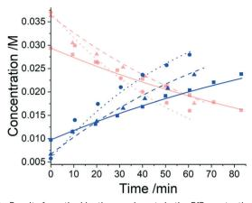
Fig. 3 Results from the kinetic experiments in the PfBr protection case study in 50:50 acetonitrile/dichloromethane, where red plots indicate PfBr concentrations and blue plots indicate Pf-Al-Me concentrations. At 30 °C: ■ = experimental data, — = ODE. At 35 °C: ▲ = experimental data, - - - = ODE. At 40 °C: • = experimental data, ····· = ODE.
