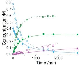
Fig. 4 Kinetic profiles for two kinetic experiments at 50 °C in methanol, with the initial concentration of maleic acid at 0.4 M and 0.8 M. At 0.4 M: • = maleic acid, — = maleic acid (ODE), ■ = monoproduct, - = mono-product (ODE),  $\triangle$  = di-product, - = di-product (ODE). At 0.8 M:  $\bigcirc$  = maleic acid, --- = maleic acid (ODE),  $\square$  = monoproduct, --- = mono-product (ODE),  $\triangle$  = di-product, --- = diproduct (ODE).
