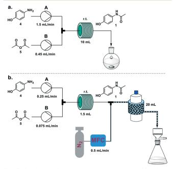
Fig. 3 Continuous flow synthesis of paracetamol (1) using a Vapourtec R2 pump module and a room temperature PFA reactor coil (10 mL, i.d. 0.8 mm). a) The product crystallized when the solution exiting the flow setup was stirred for 1 h. b) The product was crystallized inline using an SMBR system, with nitrogen introduced via a T-mixer and a 20 mL reactor (i.d. 1.6 mm) wrapped around a 1 L flask at room temperature. Crystals were collected on filter paper.
