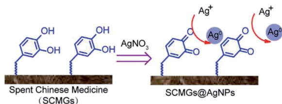
Fig. 4 A possible strategy for synthesis of SCMGs@AgNPs by using TCMs drugs.
