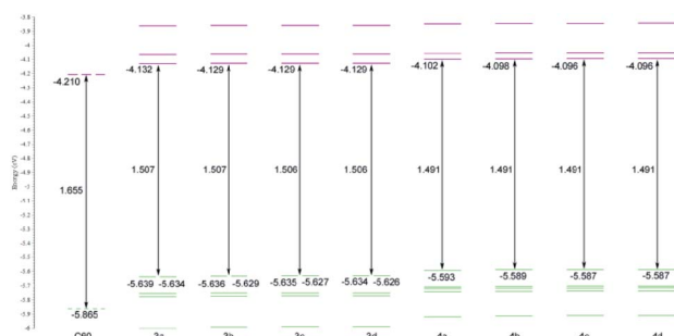
Fig. 2 Energy levels and HOMO–LUMO gaps of C_{60} and furano ( 3a–3d ) and methano ( 4a–4d ) fullerenes calculated with PBEPBE/6-311G(d,p) method. All energies are given in eV.
