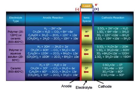
Fig. 1 Schematic illustration of the electrochemical reactions of different types of alcohol fuel-based fuel cells. Reproduced from ref. 12, Copyright 2015, Elsevier.
