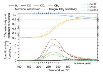
Fig. 3 MSR profiles of CZ400, CtZ600 and CmZ800 between 100 °C and 350 °C including an isothermal period of 30 min. Colour code: orange methanol conversion, blue - integral CO2 selectivity, specific activity of brown: H<sub>2</sub>, black: CO, green: CO<sub>2</sub>, grey: CH<sub>4</sub>. Heating rate: 5 °C min<sup>-1</sup>; sample mass: CZ400 - 18.6 mg, CtZ600 - 21.6 mg, CmZ800 - 20.2 mg.
