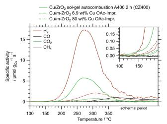
Fig. 5 Comparison of CZ400 with other impregnated Cu/ZrO<sub>2</sub> catalysts, one from literature<sup>19</sup> and another analogous system with a higher Cu loading, measured in the same recirculating batch reactor setup under identical MSR conditions
