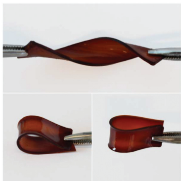
Fig. 3 Images of the cured poly(thioamide-benz-PPEO) film.
