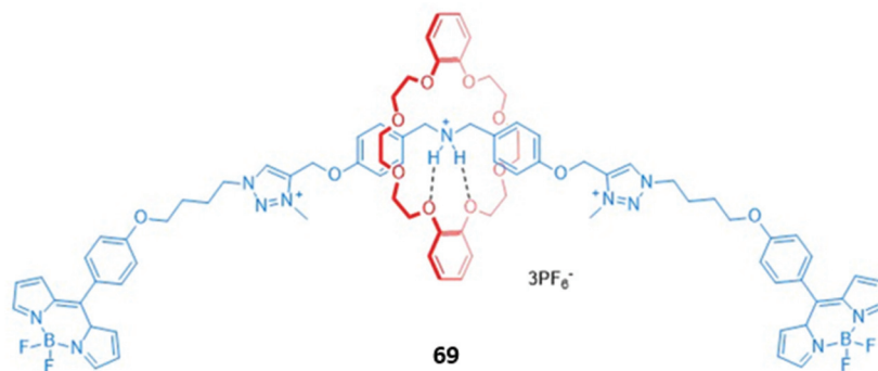
Fig. 42 A BODIPY-stoppered [2]rotaxane with a central ammonium station and peripheral imidazolium anion binding stations which binds H 2 PO 4 – ( K = 3.75 \times 10^4 \text{ M}^{-1} in CH 3 CN).
